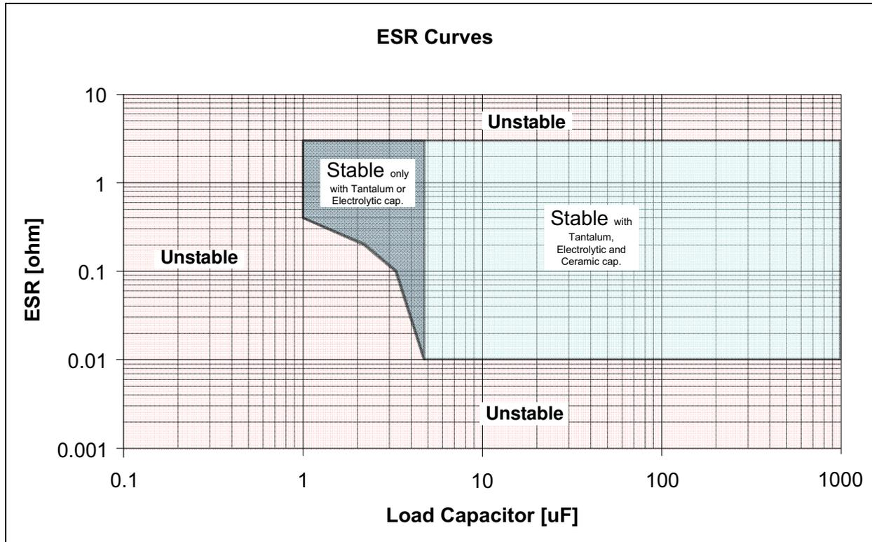
FIGURE 2-3: ESR Curves for Load Capacitor Selection.
