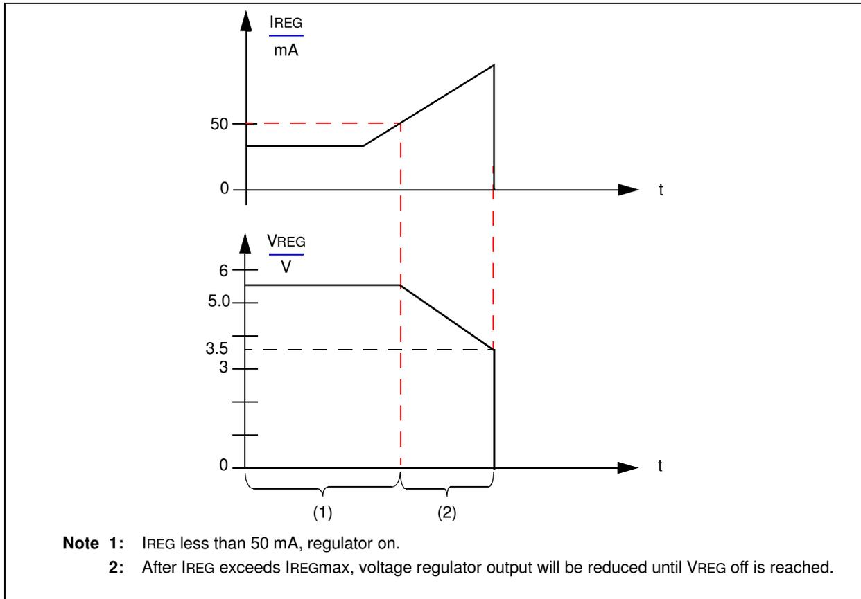
**FIGURE 1-12:** Voltage Regulator Output on Overcurrent Situation.
