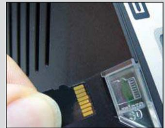
Micro smart SD card for parameterization of the i-CON pico
