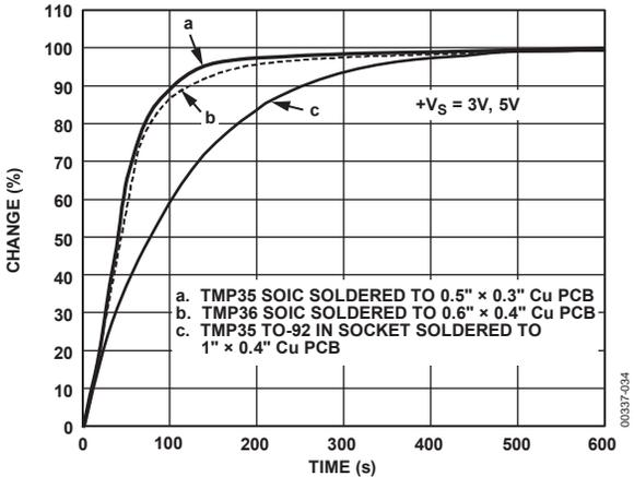
Figure 17. Thermal Response Time in Still Air
