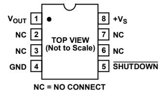
Figure 3. R-8 (SOIC\_N)
