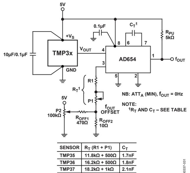
Figure 34. Temperature-to-Frequency Converter
