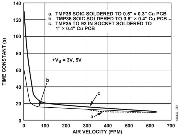
Figure 18. Thermal Response Time Constant in Forced Air
