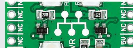
Communication lines voltage level can be in range between 1.8V and 5V. **On-board transistors** are used to drive relays by current sinking.
