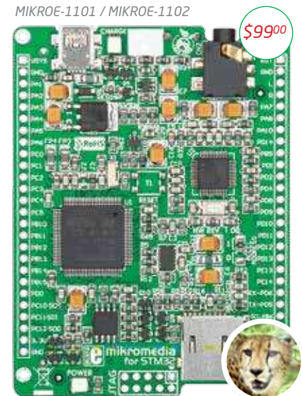
mikromedia for STM32 (features STM32F207VGT6 or STM32F407VGT6)
