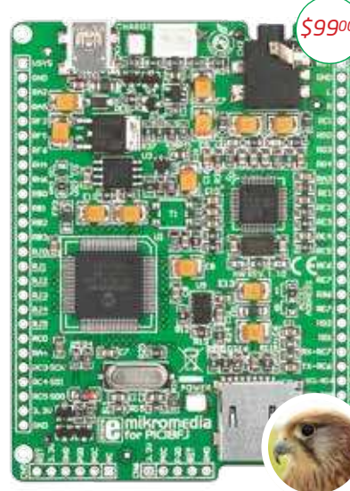
mikromedia for PIC18FJ (features PIC18F87J50)
