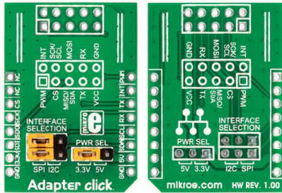
Adapter Click™ is an accessory board in **mikroBUS™** form factor. It's a compact and easy solution for adding mikroBUS™ to IDC10 adapter to your design. It features 2x5 connection pads and two jumpers for SPI/I<sup>2</sup>C selection. Adapter Click™ communicates with the target board microcontroller via **mikroBUS™** I<sup>2</sup>C (SDA, SCL), SPI (MISO, MOSI, SCK, CS), UART (RX, TX), INT and PWM lines. The board is designed to use 3.3V and 5V power supply.
