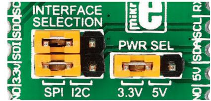
There are two jumpers for SPI/I<sup>2</sup>C selection and one used to select whether 3.3V or 5V power supply will be used.
