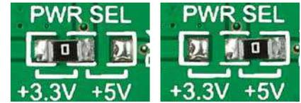
There is one zero-ohm SMD jumper **J1** used to select whether 3.3V or 5V power supply is used. Jumper **J1** is soldered in 3.3V position by default.
