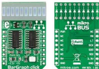
BarGraph Click™ is an accessory board in **mikroBUS™** form factor. It's a compact and easy solution for adding ten-segment light bar display to your design. It features **JSB-R102510Z** light bar display as well as two **74HC595** shift registers. BarGraph Click™ communicates with the target board microcontroller via **mikroBUS™** SPI (MOSI, MISO, SCK, CS), RST and PWM lines. The board is designed to use 3.3V and 5V power supply. LED diode (GREEN) indicates the presence of power supply.
