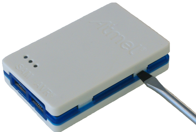
Figure 2-13. Opening the Atmel-ICE (2)
