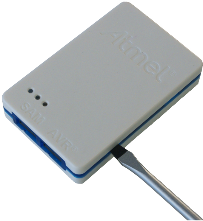
Figure 2-13. Opening the Atmel-ICE (2)
