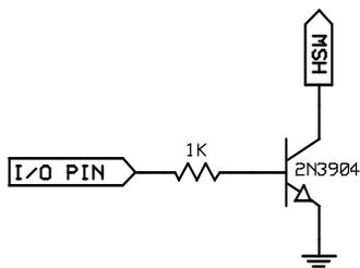
Switching circuit for the Propeller chip. Note: HIGH signal is required to turn on heater due to inversion of signal by the transistor.
