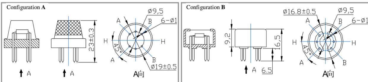
Structure and configuration of MQ-3 gas sensor is shown as Fig. 1 (Configuration A or B), sensor composed by micro  $Al_2O_3$  ceramic tube, Tin Dioxide ( $SnO_2$ ) sensitive layer, measuring electrode and heater are fixed into a crust made by plastic and stainless steel net. The heater provides necessary work conditions for work of sensitive components. The enveloped MQ-3 have 6 pin ,4 of them are used to fetch signals, and other 2 are used for providing heating current.
