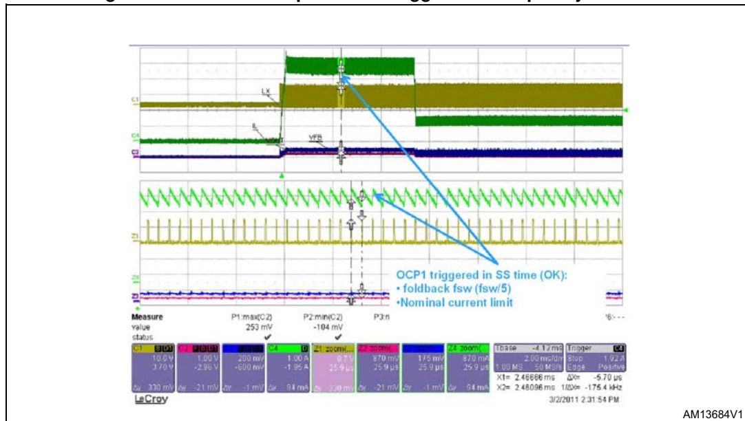
Figure 23. Over current protection triggers the frequency foldback
