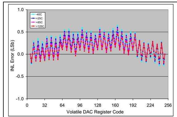
**FIGURE 2-24:** INL vs. Code (code = 6 to 250) and Temperature (MCP4706).
