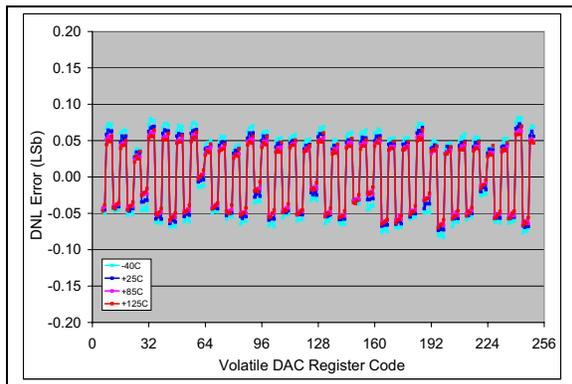
**FIGURE 2-27:** DNL vs. Code (code = 6 to 250) and Temperature (**MCP4706**).
