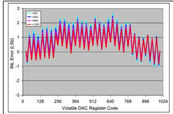
**FIGURE 2-23:** INL vs. Code (code = 25 to 1000) and Temperature (MCP4716).
