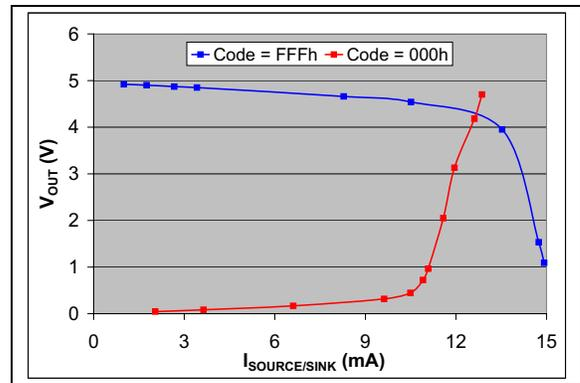
**FIGURE 2-95:**  $V_{OUT}$  vs. Source / Sink Current.  $V_{DD} = 5.0\text{V}$ .
