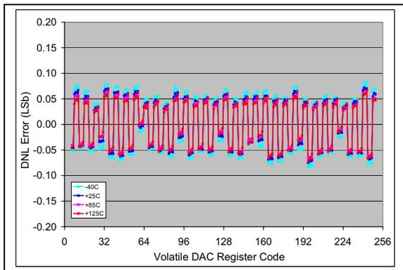
**FIGURE 2-45:** DNL vs. Code (code = 6 to 250) and Temperature (**MCP4706**).
