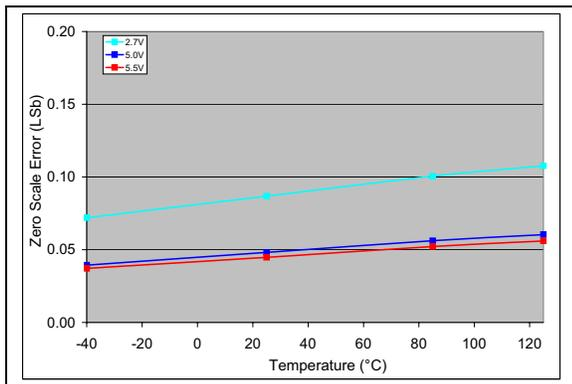
**FIGURE 2-33:** Zero Scale Error (ZSE) vs. Temperature (MCP4706).
