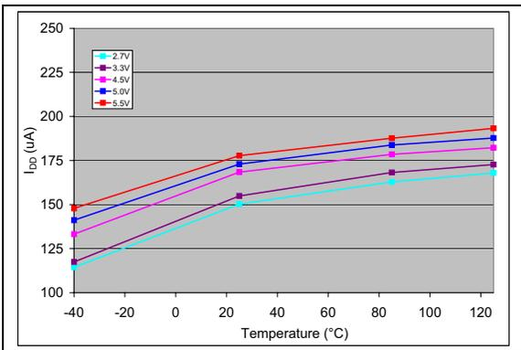
**FIGURE 2-89:**  $I_{DD}$  vs. Temperature.
