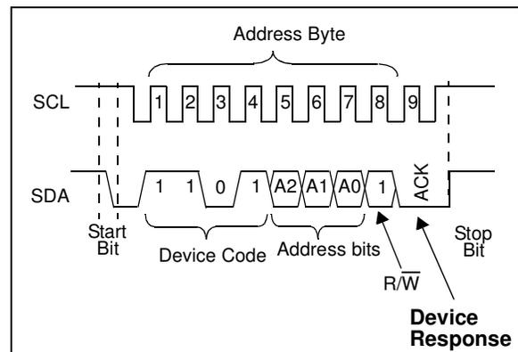
**FIGURE 8-1:** I<sup>2</sup>C Bus Connection Test.
