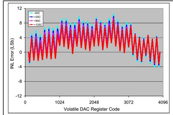
**FIGURE 2-22:** INL vs. Code (code = 100 to 4000) and Temperature (MCP4726).
