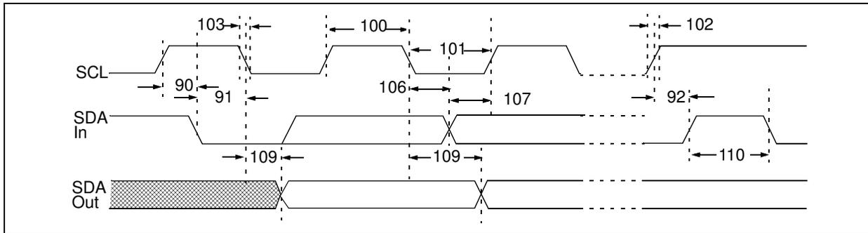
**FIGURE 1-4:** I<sup>2</sup>C Bus Data Timing.
