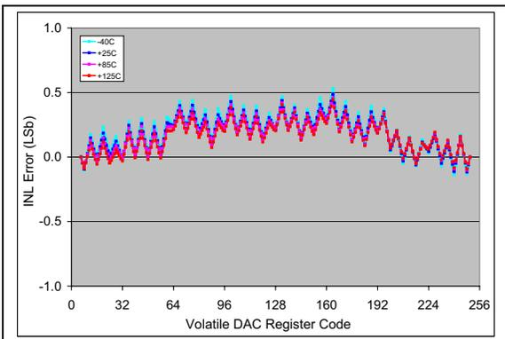
**FIGURE 2-21:** INL vs. Code (code = 6 to 250) and Temperature (MCP4706).
