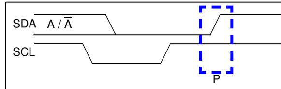
**FIGURE 5-6:** Stop Condition Receive or Transmit Mode.
