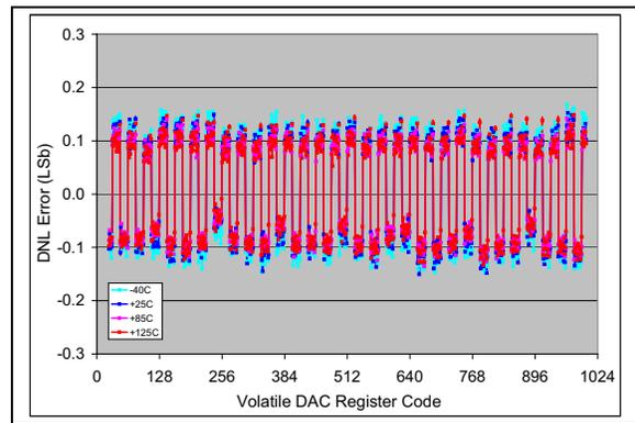
**FIGURE 2-47:** DNL vs. Code (code = 25 to 1000) and Temperature (**MCP4716**).
