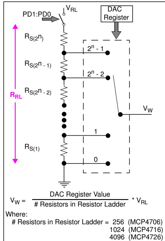
**FIGURE 4-3:** Resistor Ladder.
