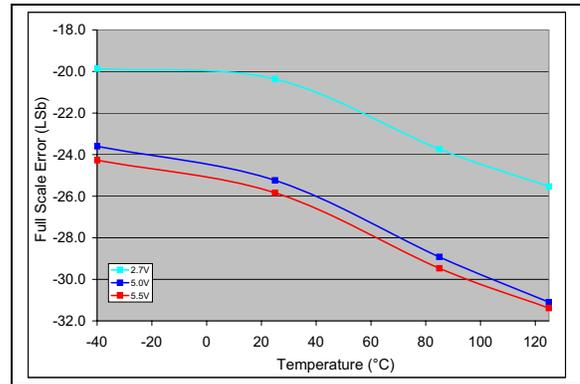
**FIGURE 2-52:** Full Scale Error (FSE) vs. Temperature (MCP4726).
