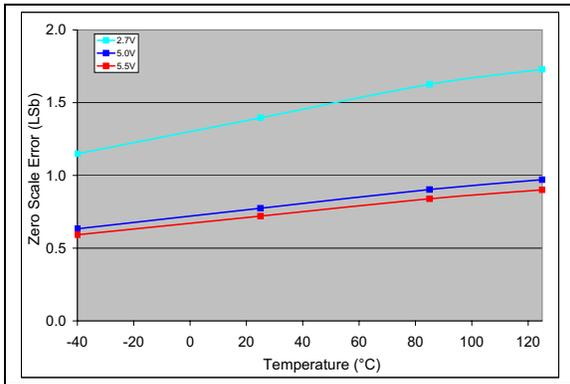
**FIGURE 2-13:** Zero Scale Error (ZSE) vs. Temperature (MCP4726).
