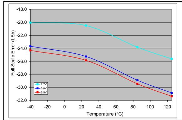
**FIGURE 2-16:** Full Scale Error (FSE) vs. Temperature (MCP4726).
