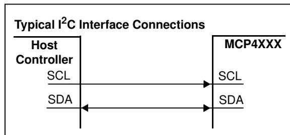
**FIGURE 5-1:** Typical I<sup>2</sup>C Interface.
