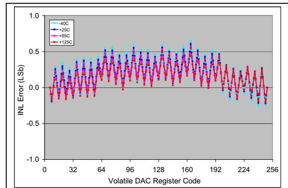
**FIGURE 2-6:** INL vs. Code (code = 6 to 250) and Temperature (MCP4706).
