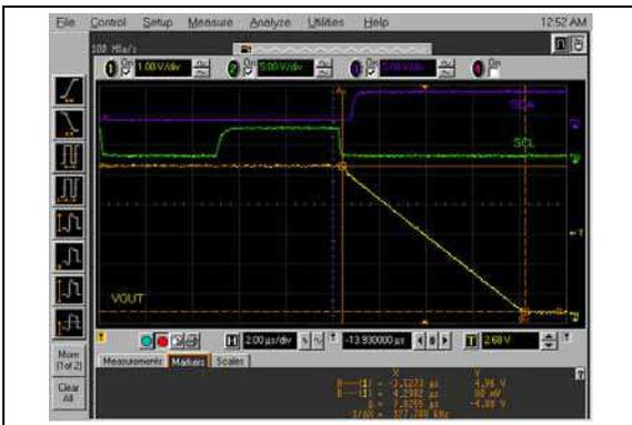
**FIGURE 2-97:** Full-Scale Settling Time (FFFh to 000h) (MCP4726).
