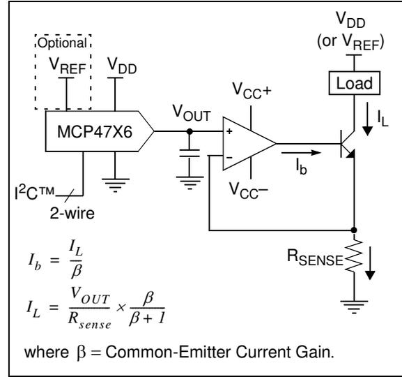
**FIGURE 8-8:** Digitally-Controlled Current Source.
