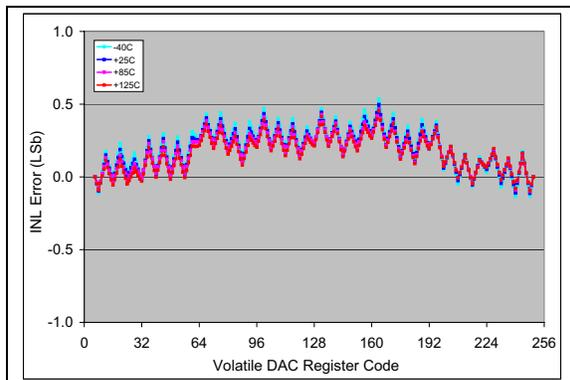
**FIGURE 2-3:** INL vs. Code (code = 6 to 250) and Temperature (MCP4706).
