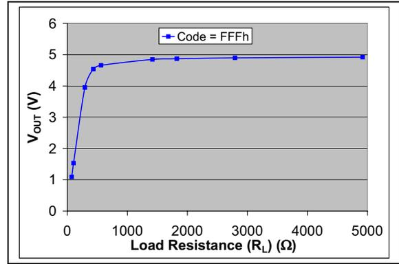
**FIGURE 2-94:**  $V_{OUT}$  vs. Resistive Load.  $V_{DD} = 5.0\text{V}$ .
