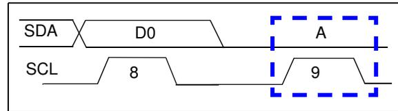
FIGURE 5-4: Acknowledge Waveform.
