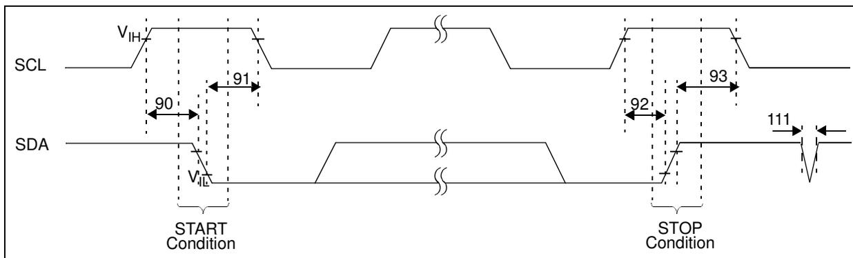
**FIGURE 1-3:** I<sup>2</sup>C Bus Start/Stop Bits Timing Waveforms.
