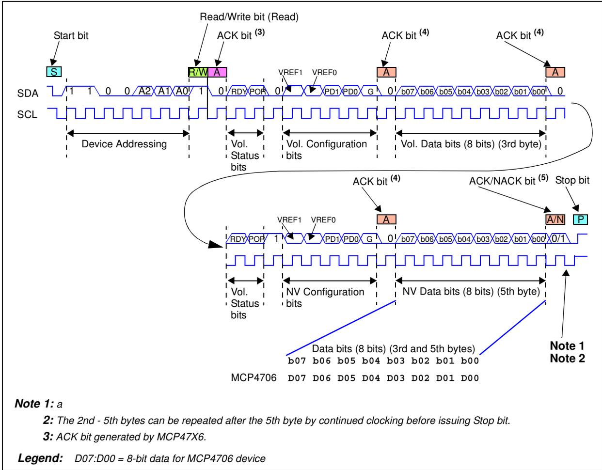
**FIGURE 6-6:** Read Command Format for 8-bit DAC (MCP4706).
