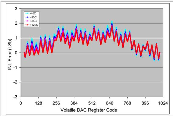
**FIGURE 2-20:** INL vs. Code (code = 25 to 1000) and Temperature (MCP4716).
