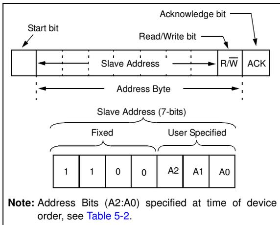
**FIGURE 5-9:** Slave Address Bits in the I<sup>2</sup>C Control Byte.
