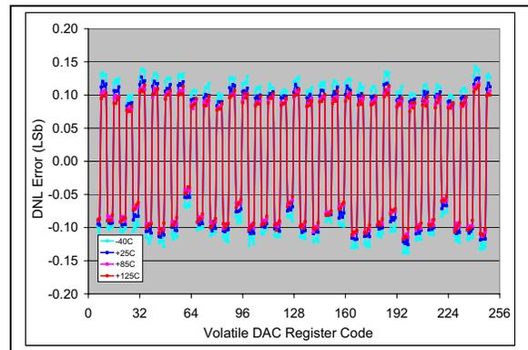
**FIGURE 2-30:** DNL vs. Code (code = 6 to 250) and Temperature (**MCP4706**).
