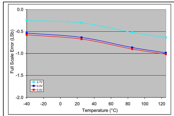
**FIGURE 2-36:** Full Scale Error (FSE) vs. Temperature (MCP4706).
