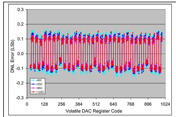
**FIGURE 2-29:** DNL vs. Code (code = 25 to 1000) and Temperature (**MCP4716**).
