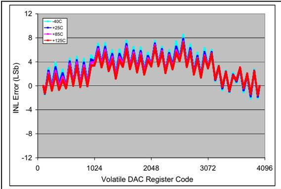
**FIGURE 2-19:** INL vs. Code (code = 100 to 4000) and Temperature (MCP4726).
