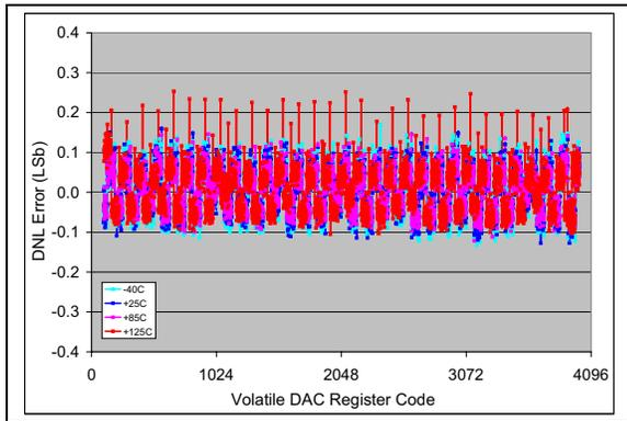
**FIGURE 2-43:** DNL vs. Code (code = 100 to 4000) and Temperature (**MCP4726**).
