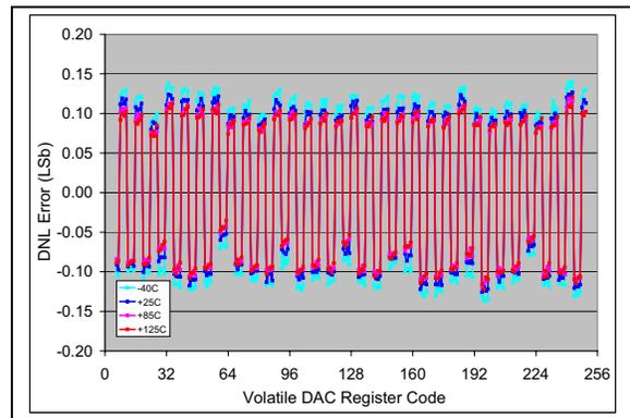
**FIGURE 2-48:** DNL vs. Code (code = 6 to 250) and Temperature (**MCP4706**).
