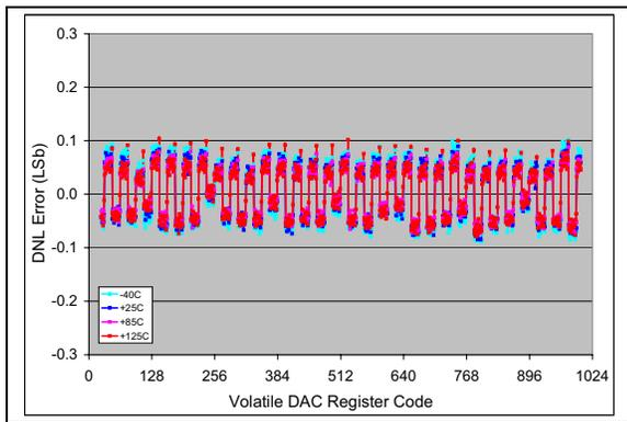
**FIGURE 2-44:** DNL vs. Code (code = 25 to 1000) and Temperature (**MCP4716**).
