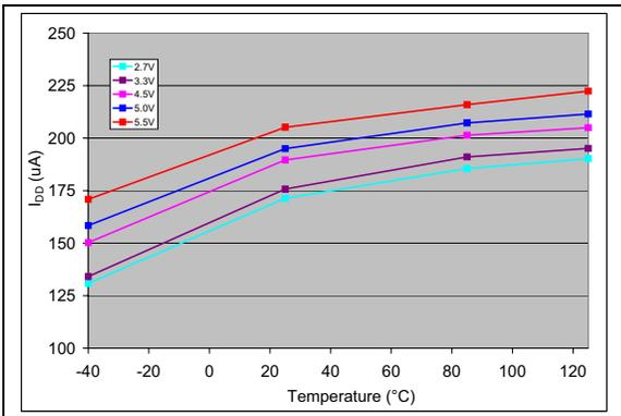
**FIGURE 2-90:**  $I_{DD}$  vs. Temperature.
