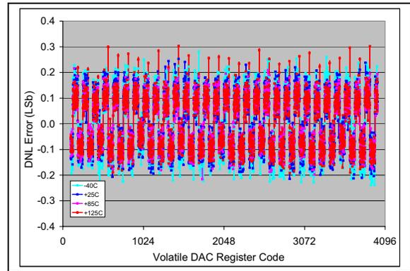
**FIGURE 2-28:** DNL vs. Code (code = 100 to 4000) and Temperature (**MCP4726**).
