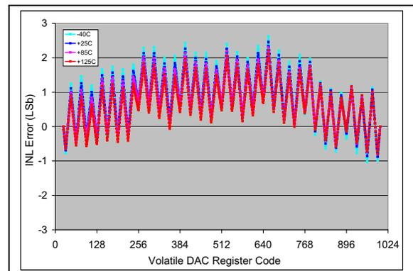
**FIGURE 2-5:** INL vs. Code (code = 25 to 1000) and Temperature (MCP4716).
