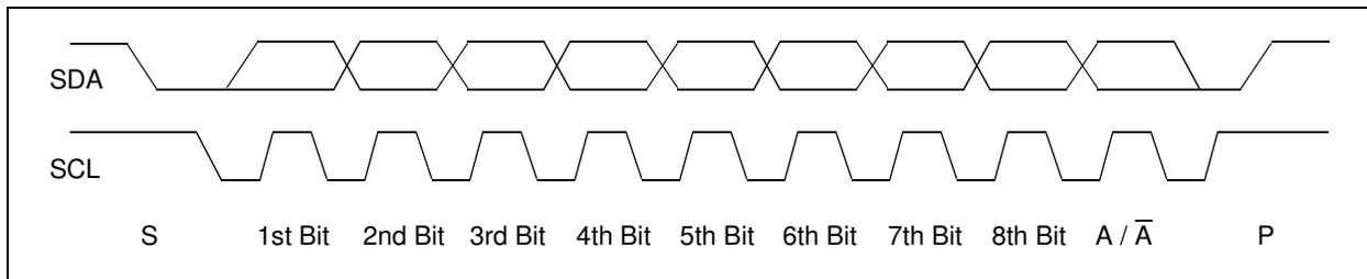
**FIGURE 5-7:** Typical 8-Bit I<sup>2</sup>C Waveform Format.
