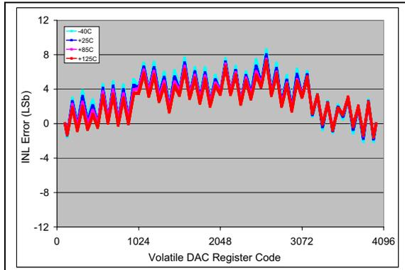
**FIGURE 2-1:** INL vs. Code (code = 100 to 4000) and Temperature (MCP4726).
