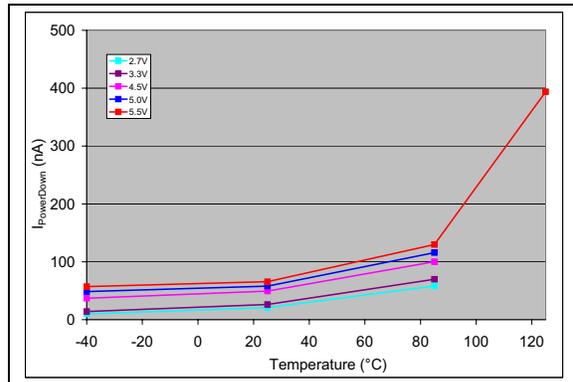
**FIGURE 2-91:** Powerdown Current vs. Temperature.
