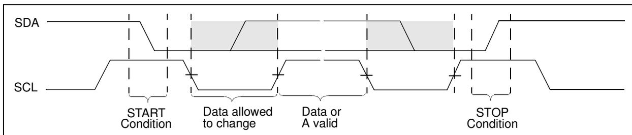
**FIGURE 5-8:** I<sup>2</sup>C Data States and Bit Sequence.
