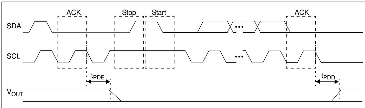
**FIGURE 1-2:** I<sup>2</sup>C Power-Down Command Timing.
