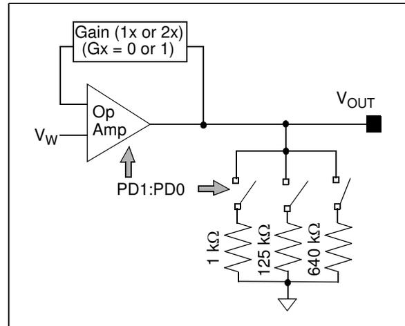
**FIGURE 4-5:** Op Amp to  $V_{OUT}$  Pin Block Diagram.
