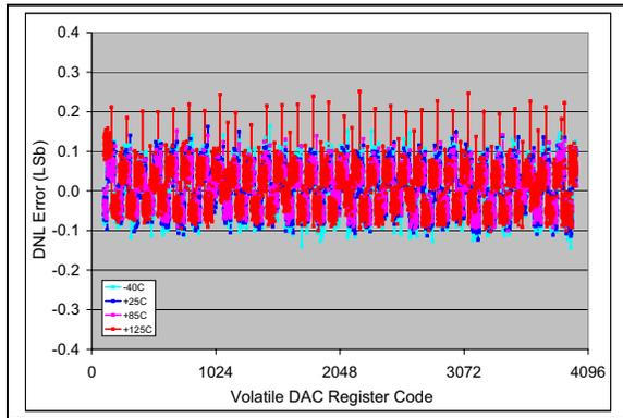
**FIGURE 2-25:** DNL vs. Code (code = 100 to 4000) and Temperature (**MCP4726**).
