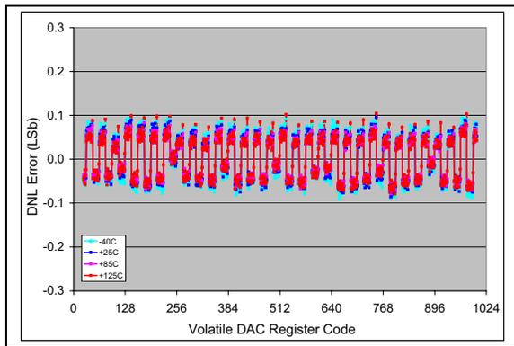
**FIGURE 2-26:** DNL vs. Code (code = 25 to 1000) and Temperature (**MCP4716**).
