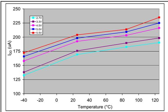
**FIGURE 2-88:**  $I_{DD}$  vs. Temperature.
