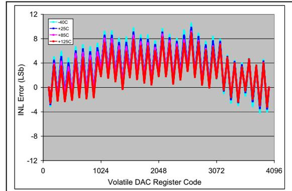
**FIGURE 2-4:** INL vs. Code (code = 100 to 4000) and Temperature (MCP4726).
