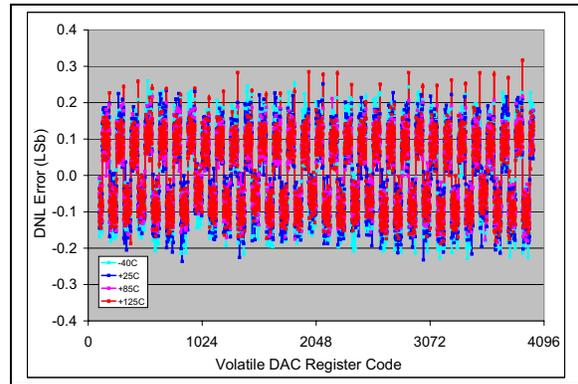
**FIGURE 2-46:** DNL vs. Code (code = 100 to 4000) and Temperature (**MCP4726**).
