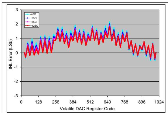
**FIGURE 2-2:** INL vs. Code (code = 25 to 1000) and Temperature (MCP4716).
