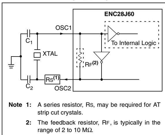
**FIGURE 2-2: EXTERNAL CLOCK SOURCE<sup>(1)</sup>**
