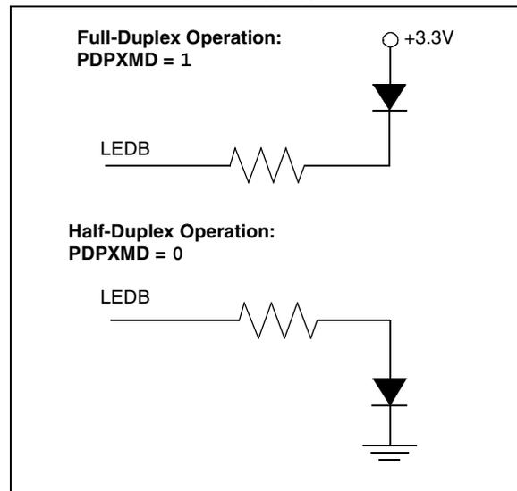
The LEDs can also be configured separately to control their operating polarity (on or off when active), blink rate and blink stretch interval. The options are controlled by the LACFG3:LACFG0 and LBCFG3:LBCFG0 bits. Typical values for blink stretch are listed in Table 2-1.
