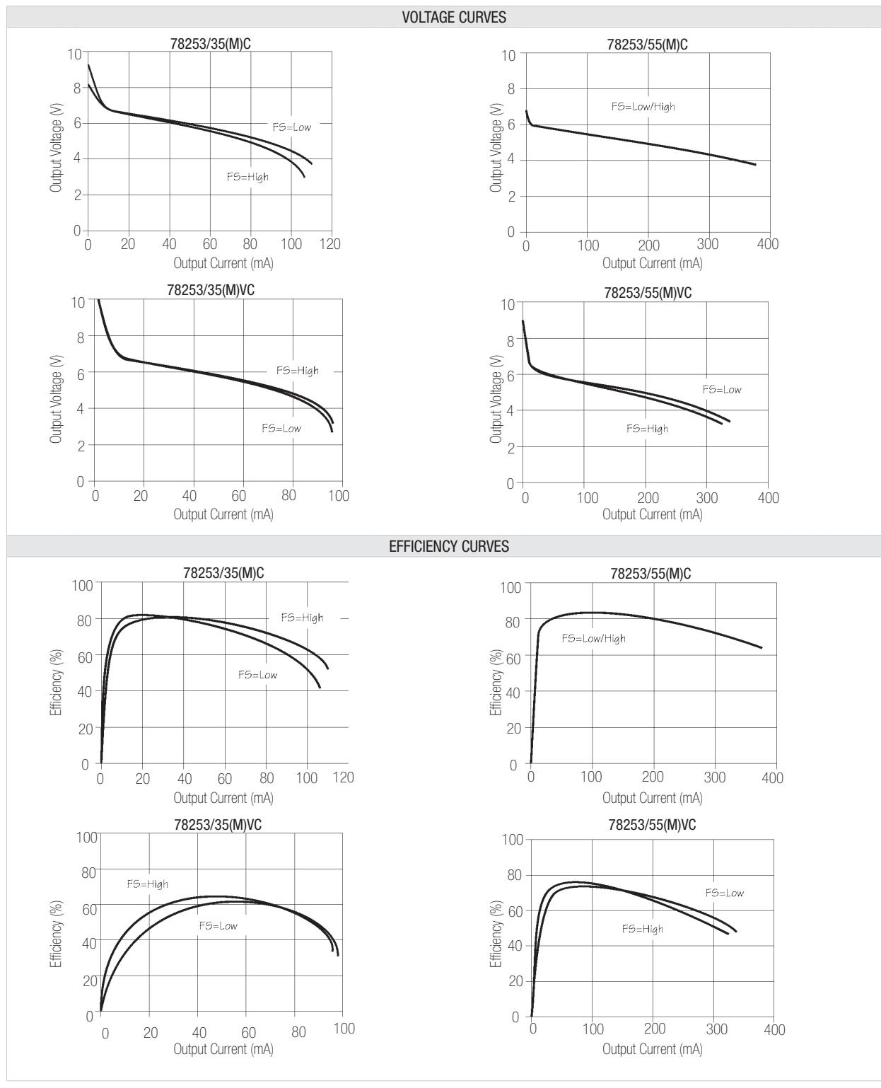
All curves are derived from testing with the Maxim MAX253 IC using the circuit shown in application note MPAN-03 ( download at <http://www.murata-ps.com/data/apnotes/mpan-03.pdf>).
