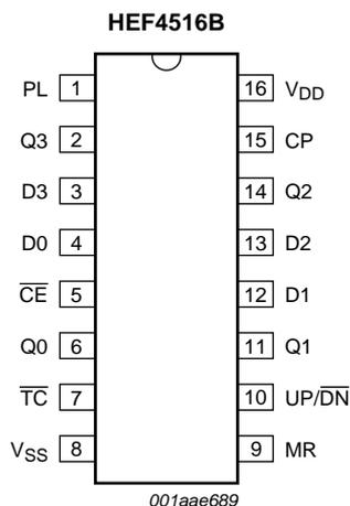
Fig 3. Pin configuration
