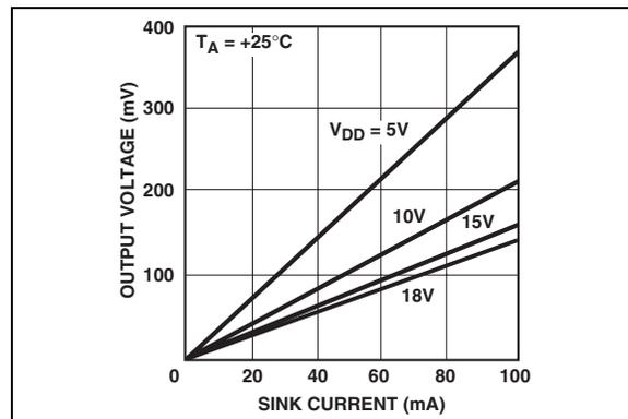
**FIGURE 2-12:** Low Output Voltage vs. Output Sink Current.
