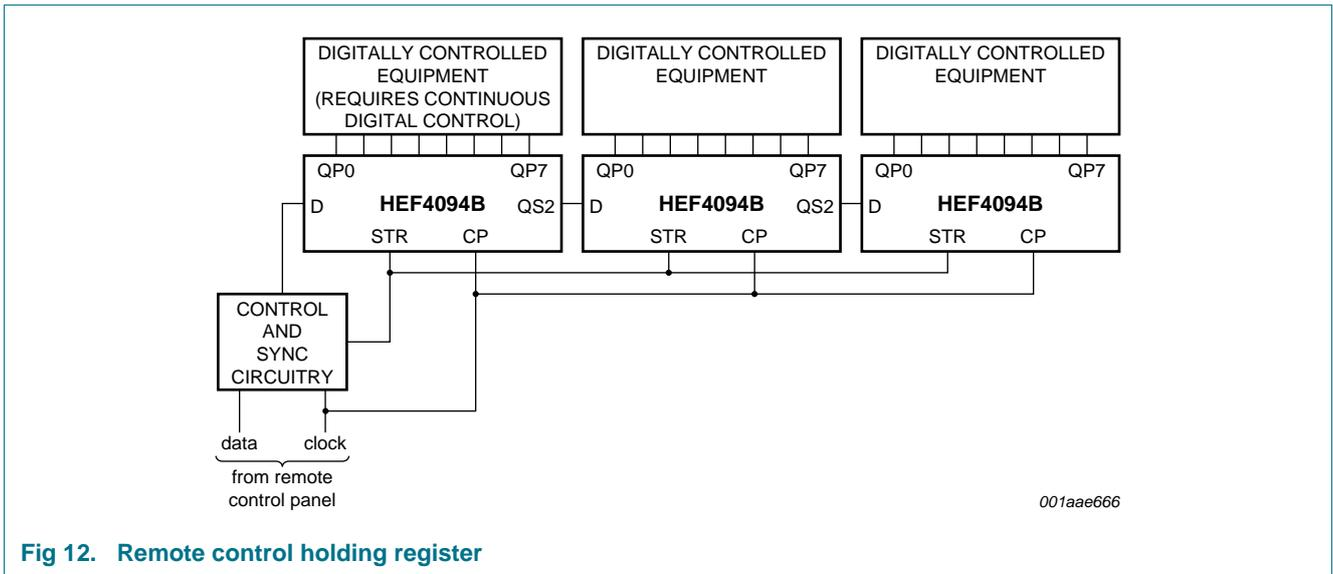
Fig 12. Remote control holding register
