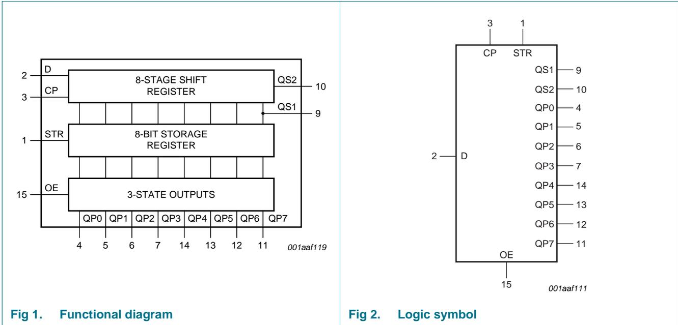
Fig 1. Functional diagram
