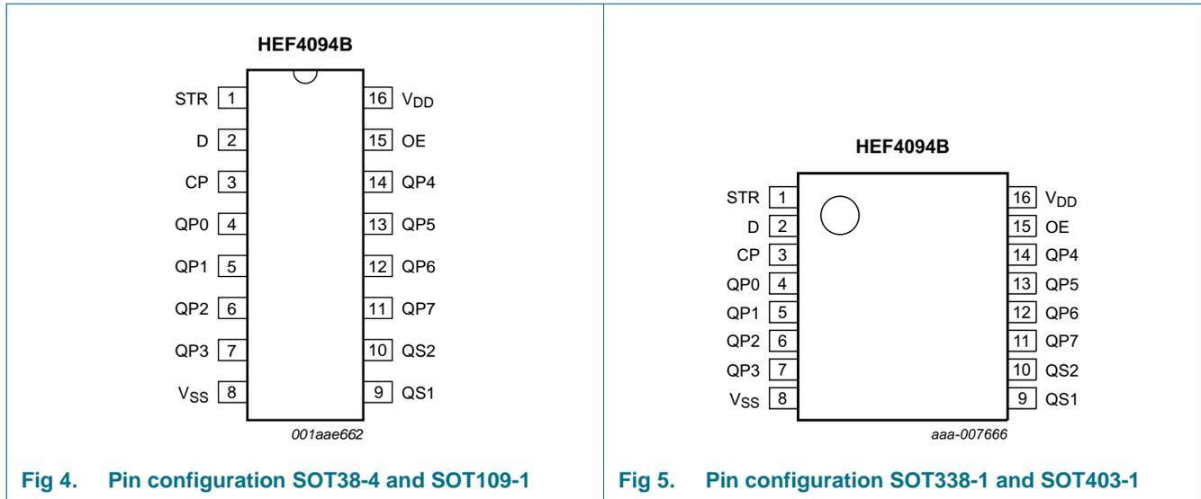
Fig 4. Pin configuration SOT38-4 and SOT109-1
