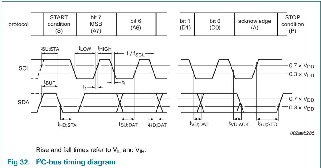
Fig 32. I<sup>2</sup>C-bus timing diagram
