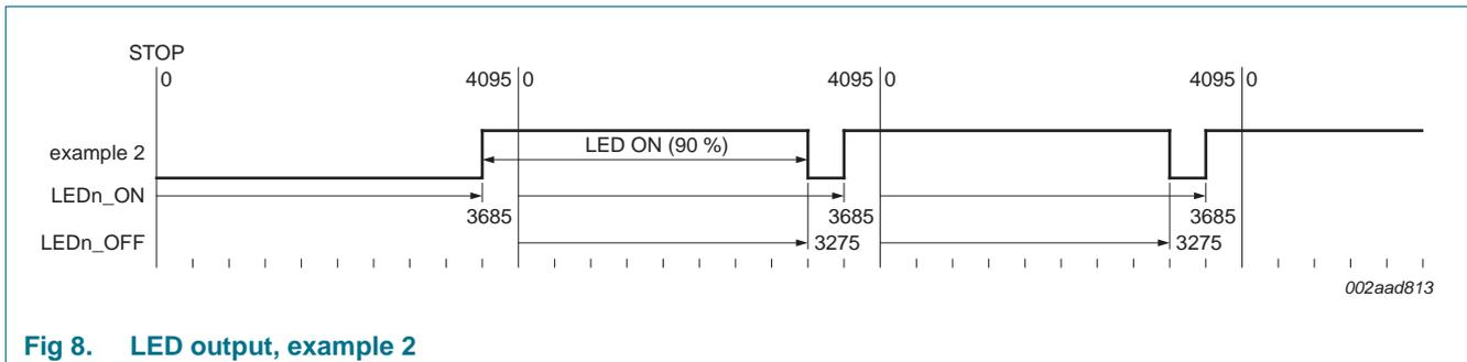
Fig 8. LED output, example 2
