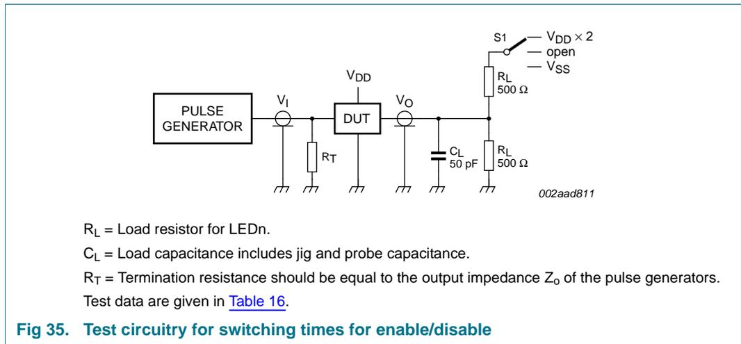
**Table 16. Test data for enable/disable switching times**
