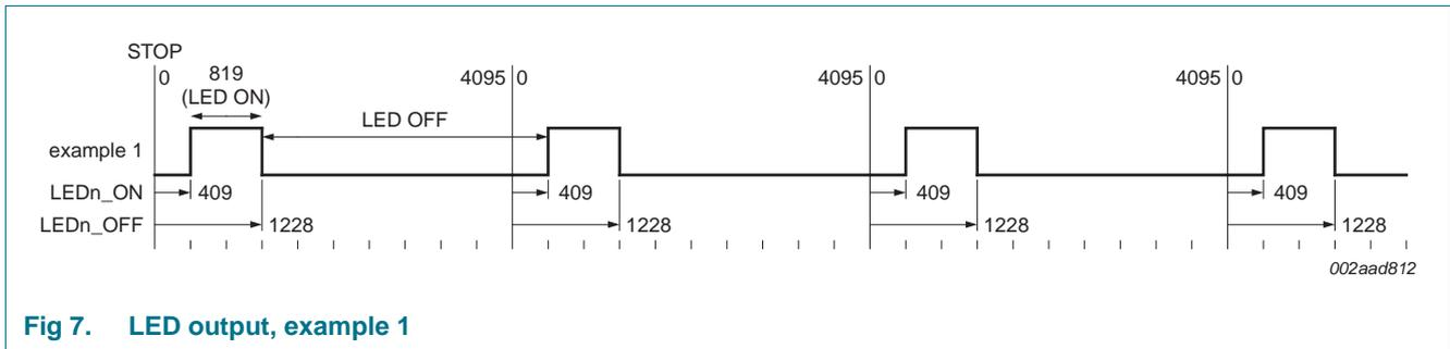
Fig 7. LED output, example 1
