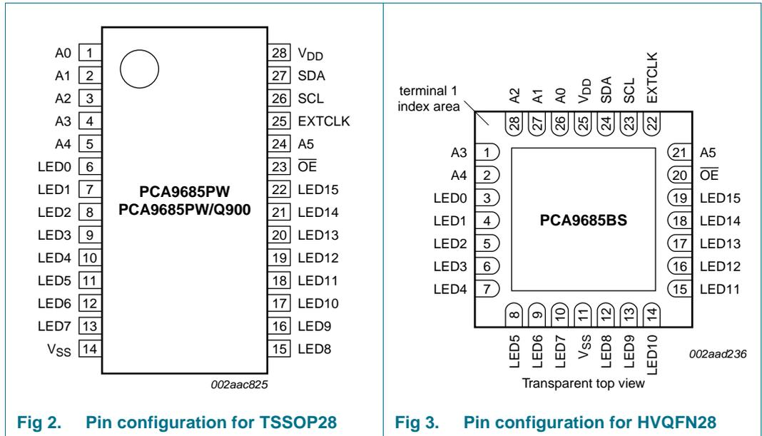
Fig 2. Pin configuration for TSSOP28
