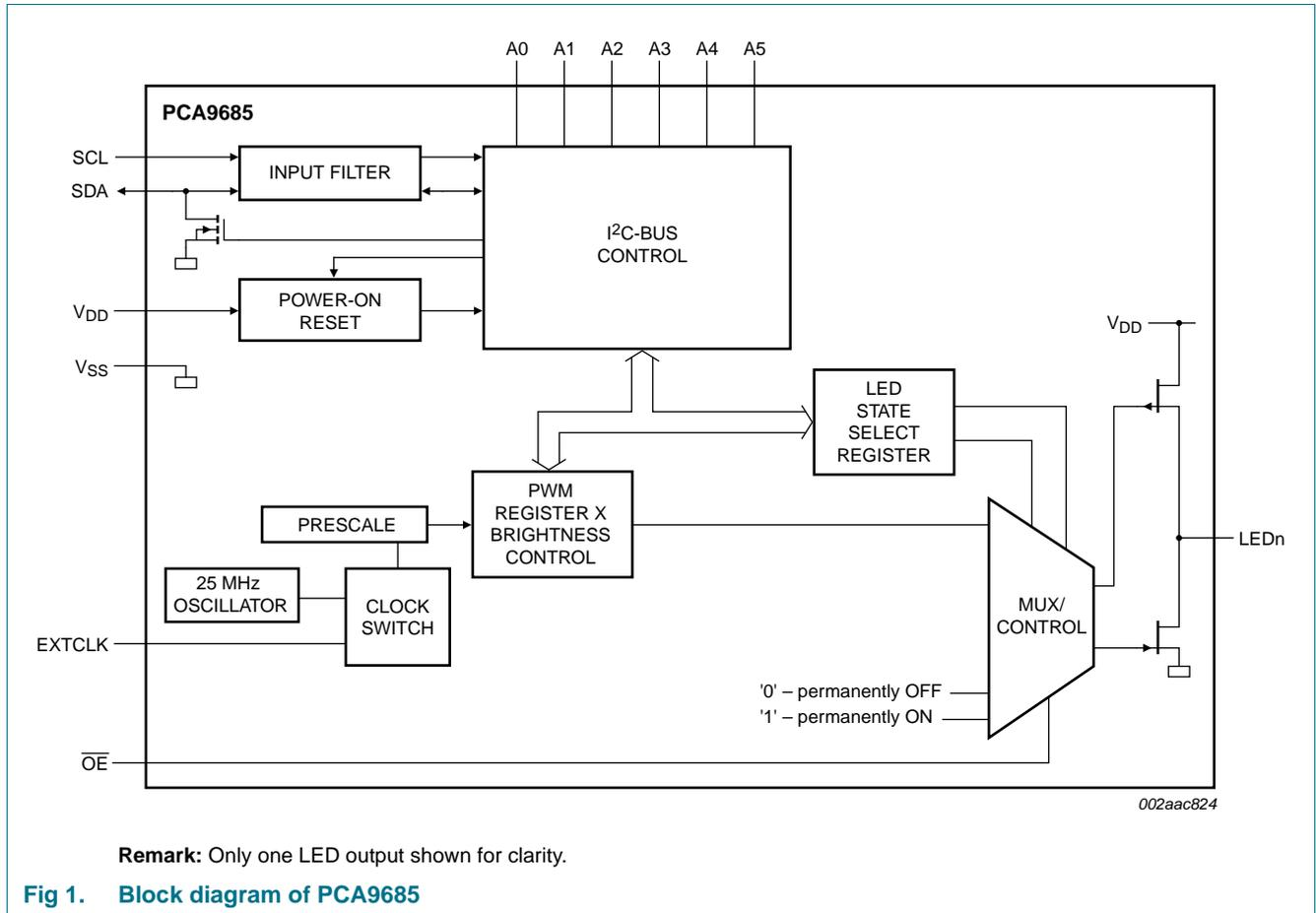
Fig 1. Block diagram of PCA9685
