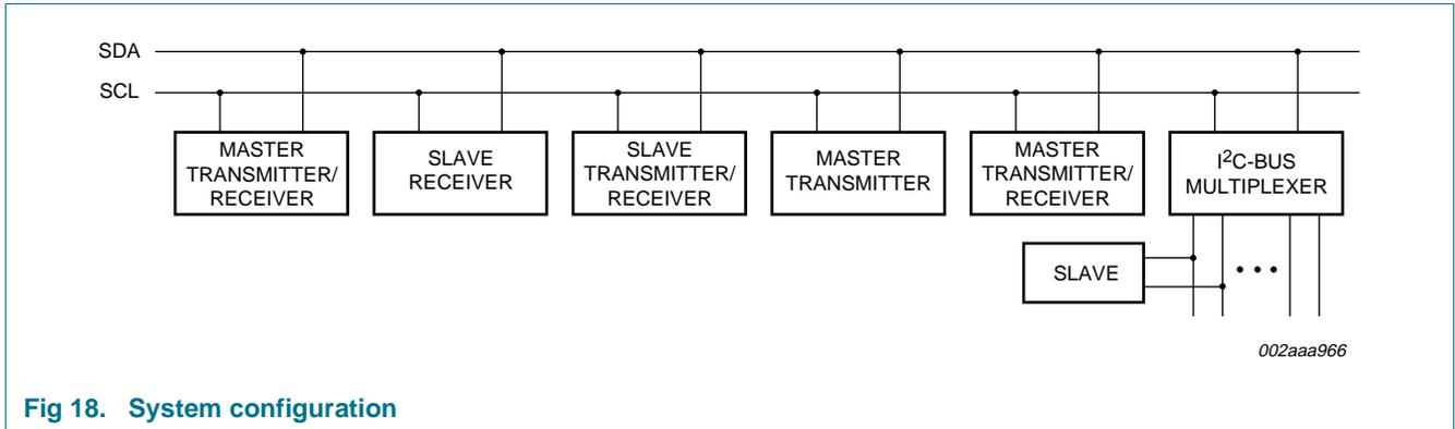
Fig 18. System configuration
