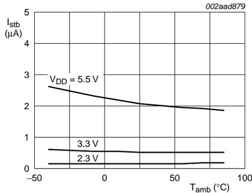
**Fig 30. Standby supply current versus temperature**
