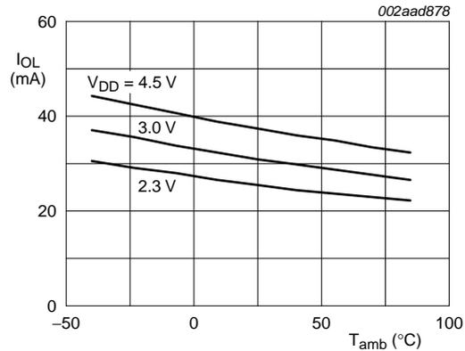
**Fig 29.  $I_{OL}$  typical drive (LEDn outputs) versus temperature**
