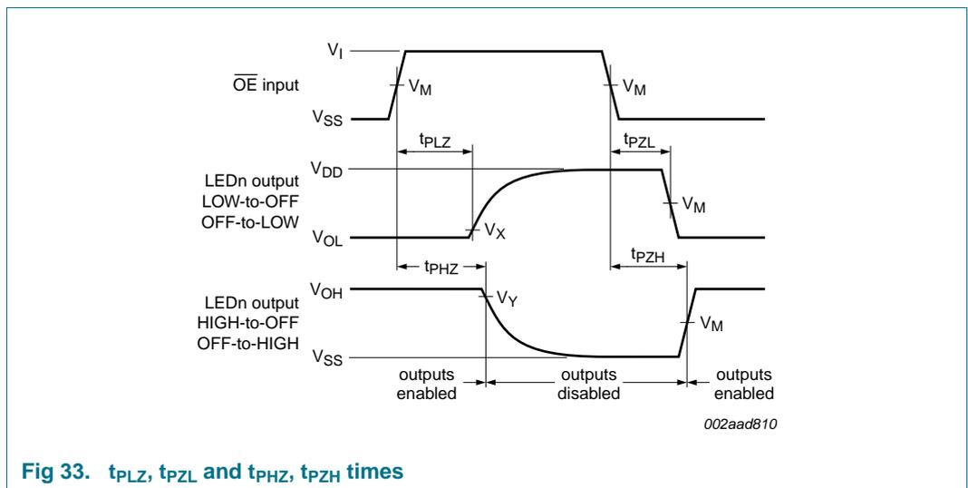
Fig 33.  $t_{PLZ}$ ,  $t_{PZL}$  and  $t_{PHZ}$ ,  $t_{PZH}$  times
