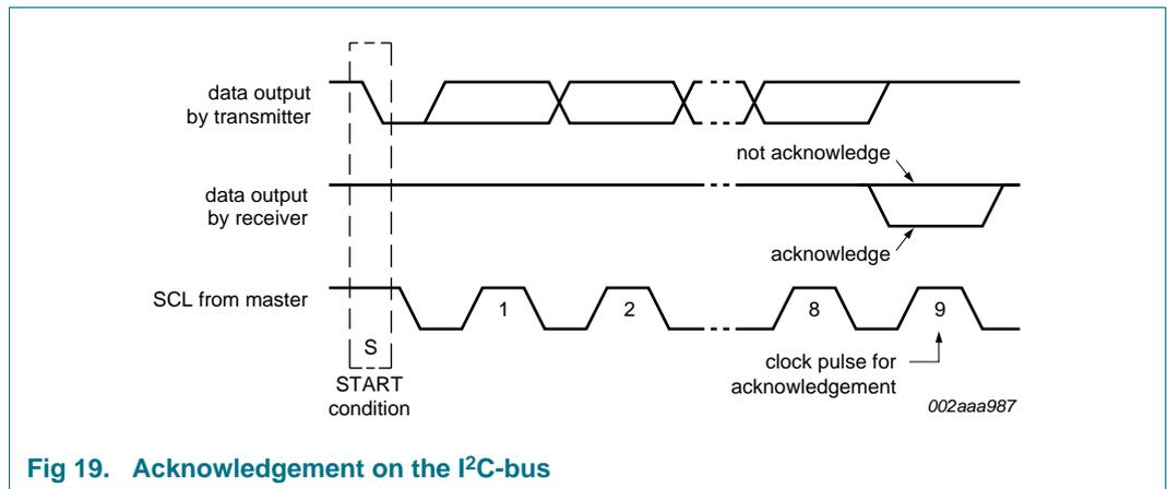
Fig 19. Acknowledgement on the I<sup>2</sup>C-bus
