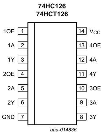
Fig 4. Pin configuration for SOT27-1 and SOT108-1
