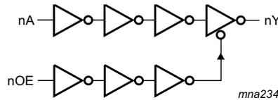
Fig 3. Logic diagram (one buffer/line driver)
