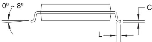
Note: 1. Dimensions D and E1 do not include mold Flash or protrusion. Mold Flash or protrusion shall not exceed 0.25 mm (0.010").
