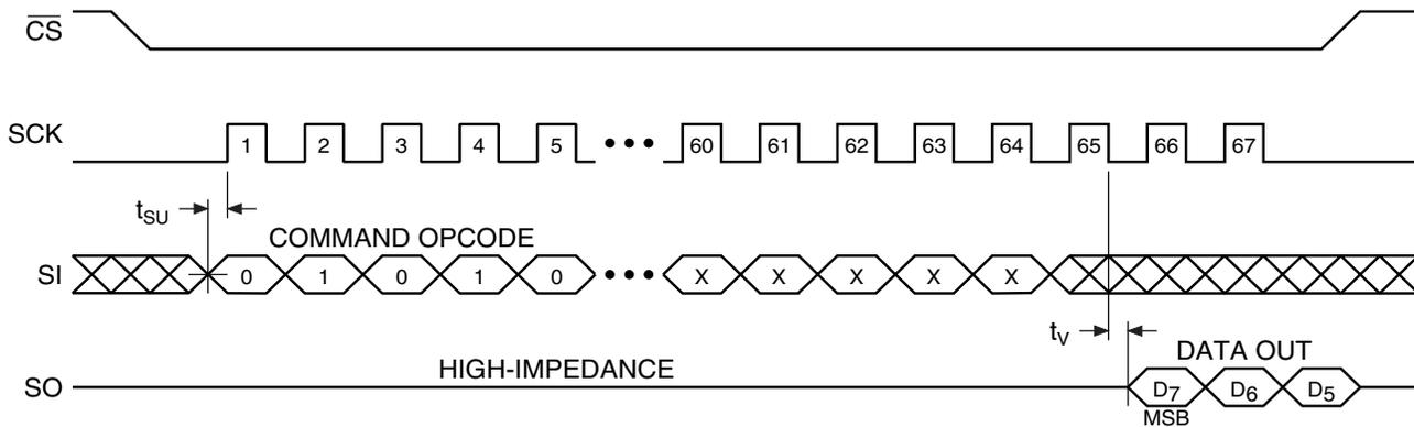
Detailed Bit-level Read Timing – Inactive Clock Polarity Low (Continued)
