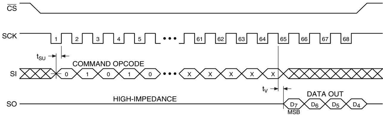
Detailed Bit-level Read Timing – Inactive Clock Polarity High (Continued)
