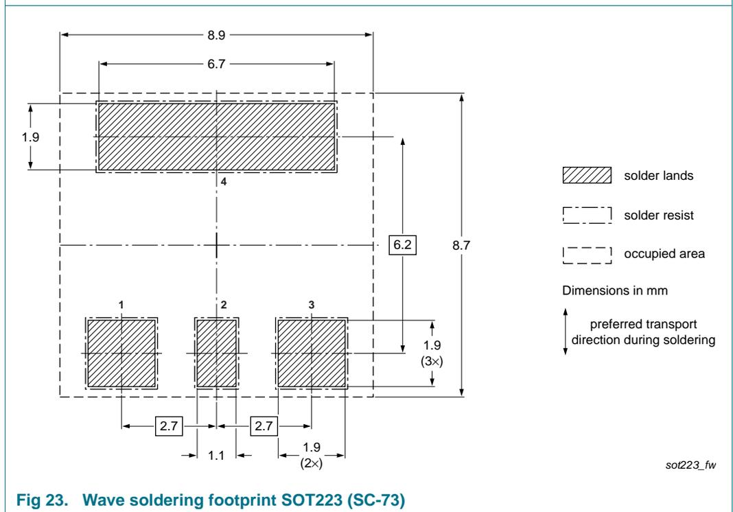
**Fig 23. Wave soldering footprint SOT223 (SC-73)**
