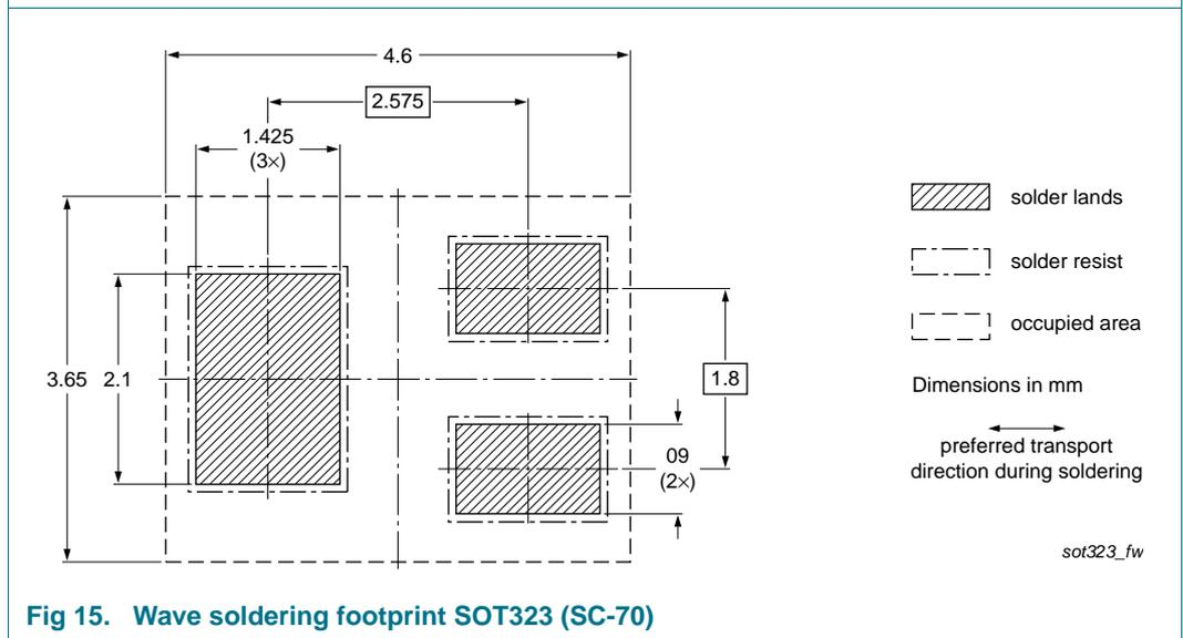
Fig 15. Wave soldering footprint SOT323 (SC-70)
