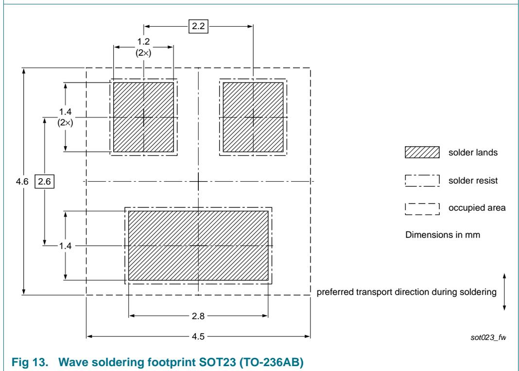
Fig 13. Wave soldering footprint SOT23 (TO-236AB)
