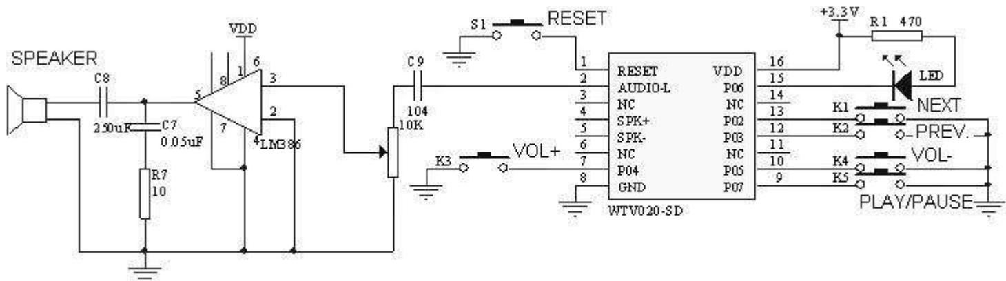
WTV020-SD-16P DAC output," Audio L" and module GND to amplifier. WTV020-SD-20S DAC output, "SPK+" and module GND to amplifier.
