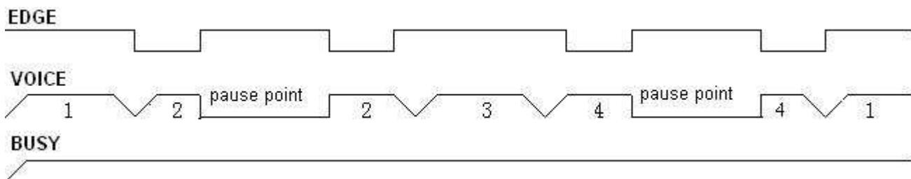
Negative edge trigger. Power on , it will play automatically, negative edge trigger P04 to pause , next tirgger to play from the pause point. After voices play finished, it will loop .
