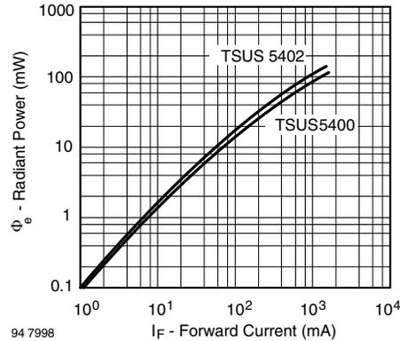
Fig. 7 - Radiant Power vs. Forward Current
