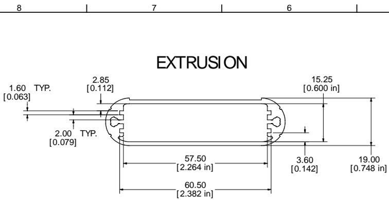
Extrusion designed for 60mm wide x 80mm long PCBs.
