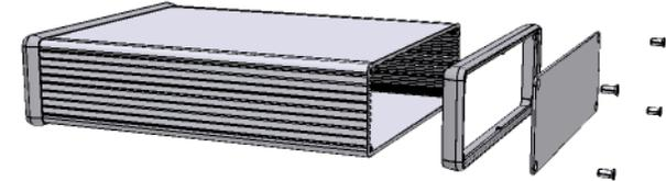
EXTRUSION DESIGNED FOR 160MM WIDE PC BOARD
