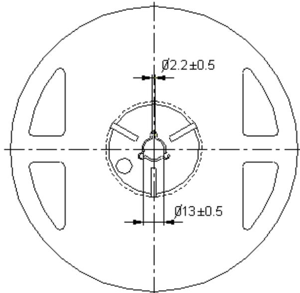
Note: 01. The tolerance unless mentioned is  $\pm 0.1$ mm
