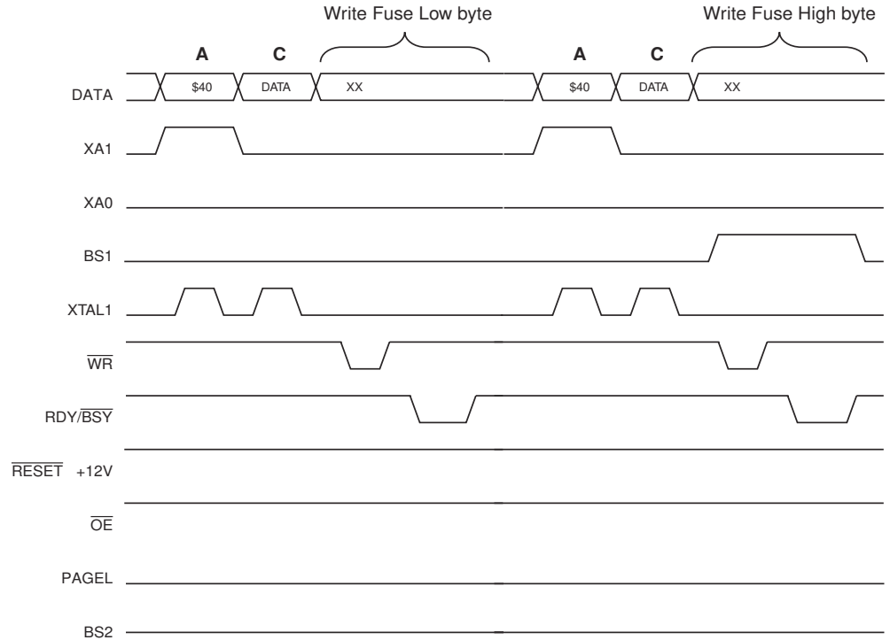
Figure 79. Programming the Fuses Waveforms
