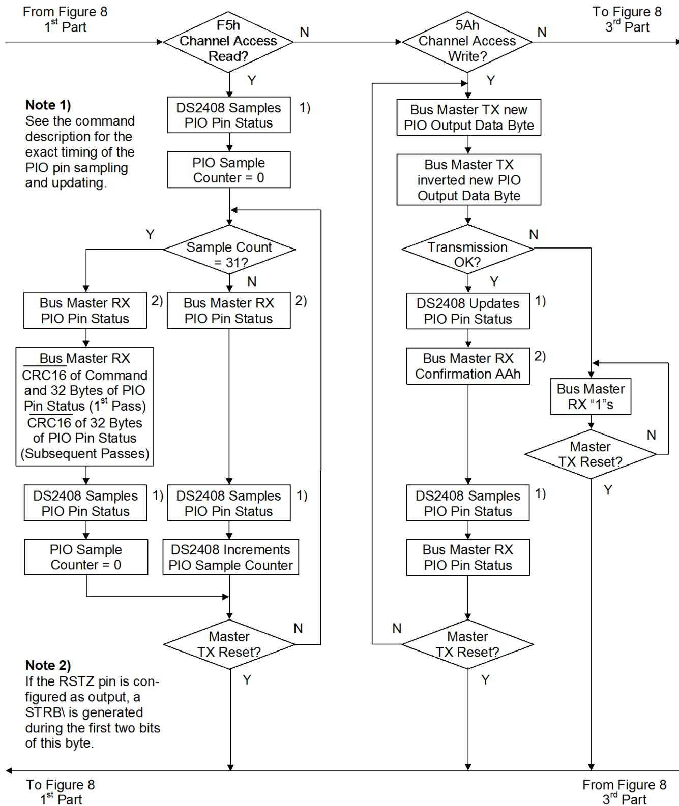
**Figure 8-3. CONTROL FUNCTIONS FLOW CHART**
