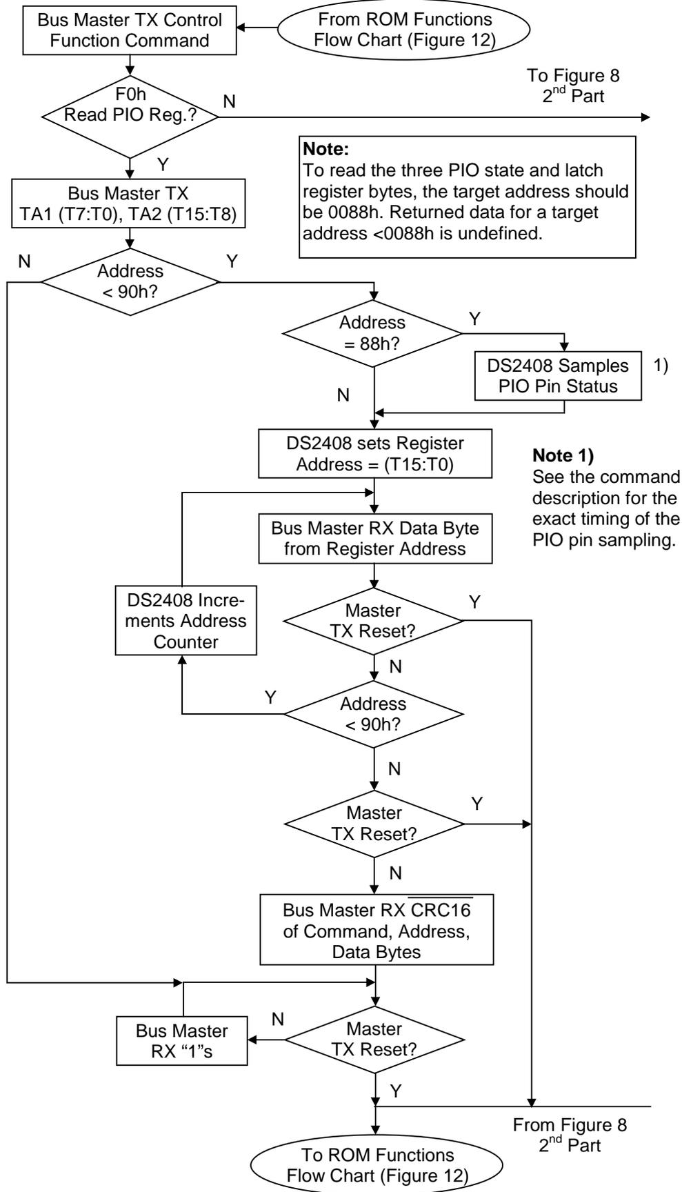
**Figure 8-2. CONTROL FUNCTIONS FLOW CHART**
