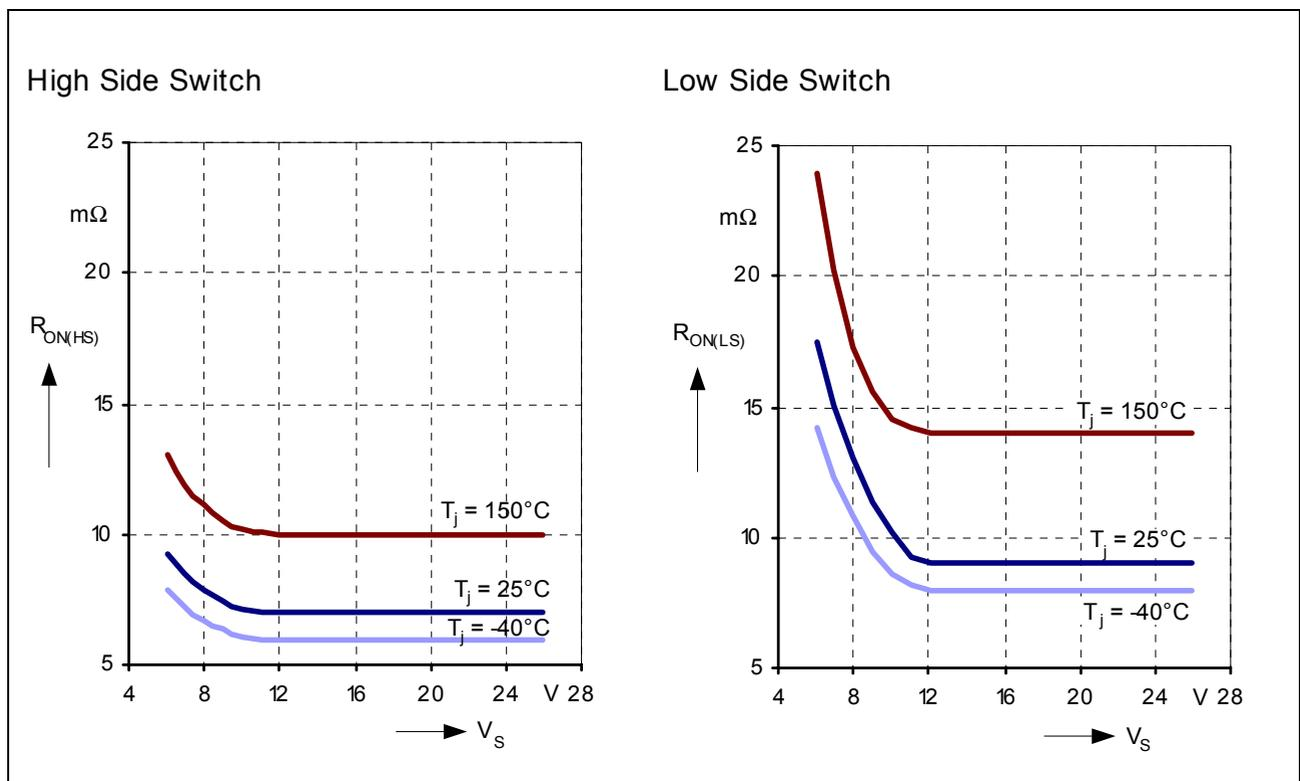
**Figure 4** Typical On State Resistance vs. Supply Voltage
