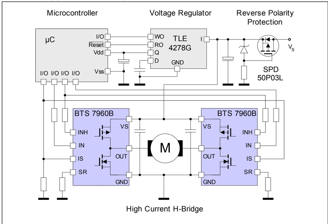
**Figure 11 Application Example: H-Bridge with two BTS 7960B**
