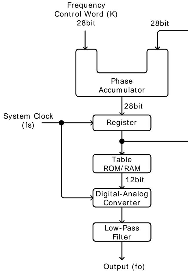
The phase accumulator adds the frequency control word K at every clock cycle  $f_s$ . The accumulator output points to a location in the Table ROM/RAM. The DAC converts the digital data into an analog waveform. The LPF filters out the clock frequency to provide a pure waveform.
