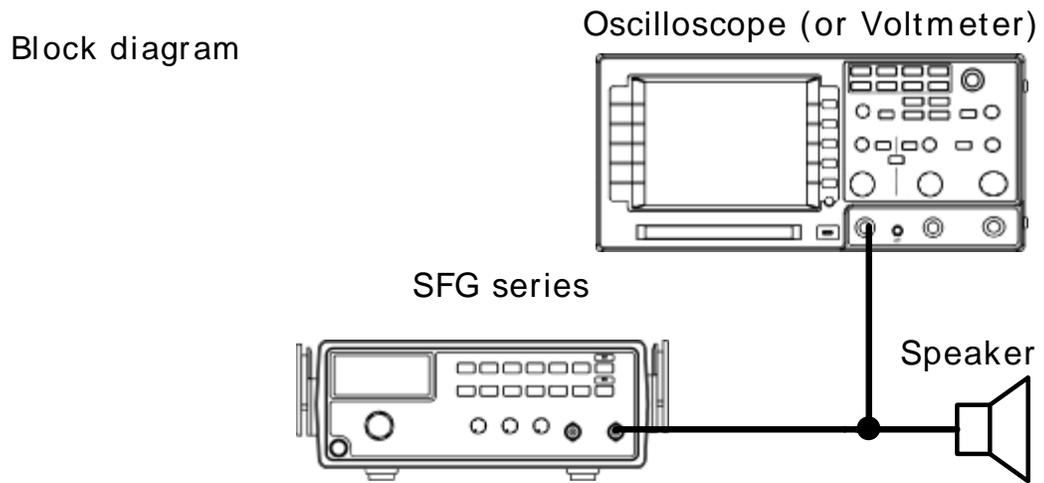
**Graph** The peak voltage occurs on the resonant frequency of the speaker.
