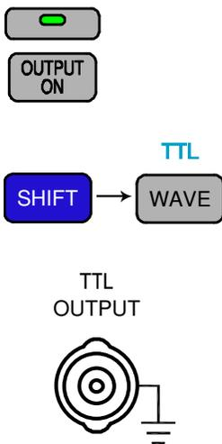
1. Press the Output key. The LED turns On. (TTL does not activate unless the output is already On)
