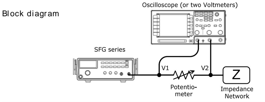
**Test step** Adjust the potentiometer until V2 becomes the half of V1 ( $V2=0.5V1$ ). Then the impedance Z of the network becomes identical to the potentiometer.
