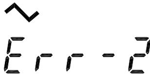
Triangle waveform frequency is limited to maximum 1MHz. When the input exceeds it, an error message (Err-2) appears and forces the frequency to 1MHz.
