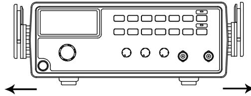
Pull out the handle sideways and rotate it.
