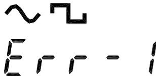
Sine and square waveform frequency is limited to maximum 3MHz. When the input exceeds it, an error message (Err-1) appears and forces the frequency to 3MHz.
