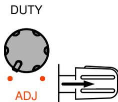
Pull out the Duty knob. Turn right (left) to increase (decrease) the duty cycle. The default is set at 50%.
