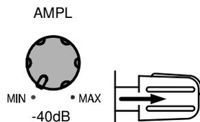
Pull out the Amplitude knob. The output amplitude is attenuated by -40dB.
