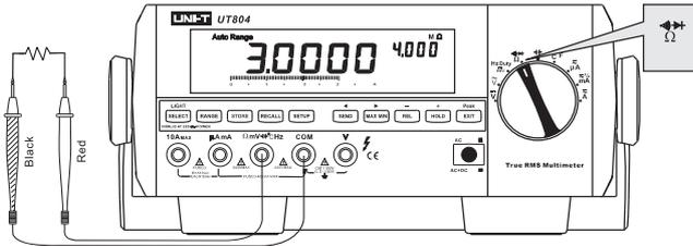
Figure 3-10. Resistance Measurement
