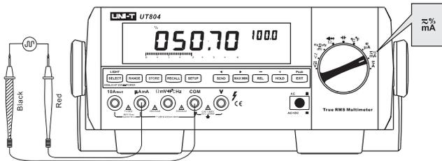
Figure 3-16. 4~20mA loop current as % readout
