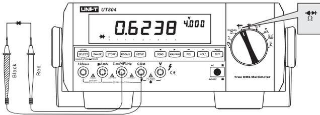
Figure 3-12. Diode Test
