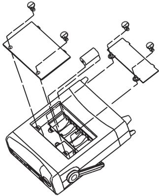
Figure 6-2. Battery Replacement
