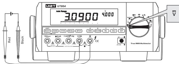
Figure 3-1. DC Voltage Measurement
