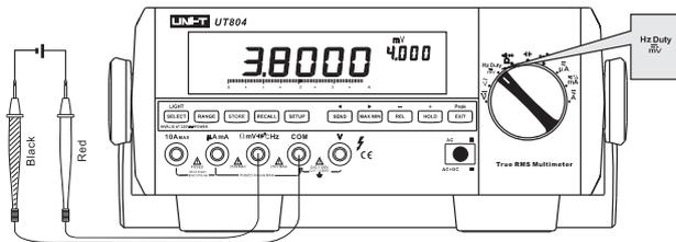
Figure 3-3. DC Millivoltage Measurement
