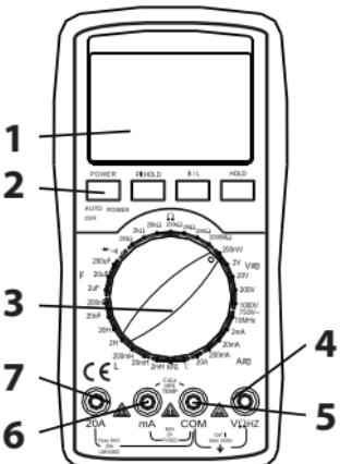
**1.** LCD: displays the measured value and unit
